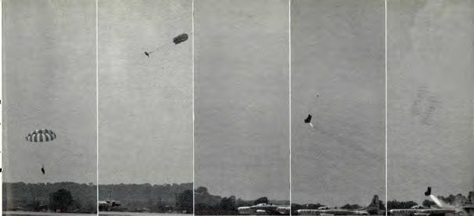
Long overdue is a zero altitude escape system. Here is one using rocket catapult, seat/man separator, and I and I second timing system. Extreme right, seat clears the '94; on the way up; top of trajectory and seat separation; parachute blossoms; and finally the successful descent.
