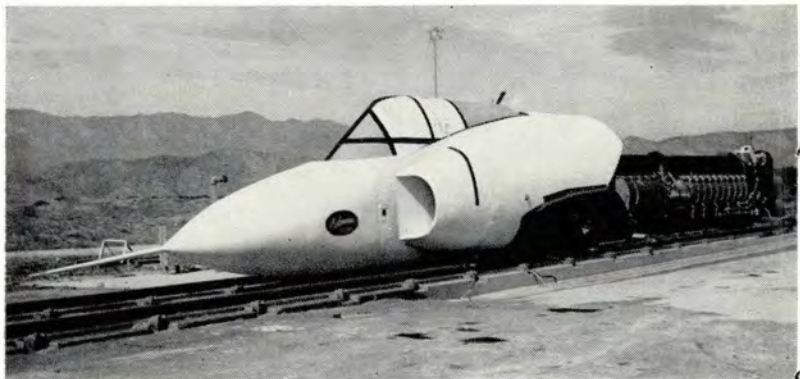
Experimental pod or canopy capsule is shown on sled prior to track test.
