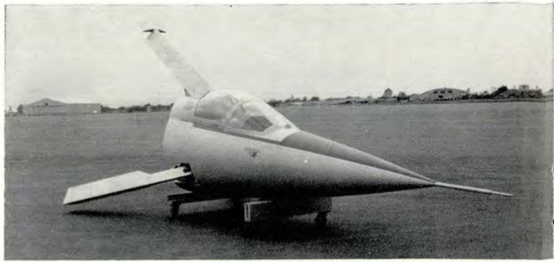
Mockup of experimental nose type capsule. Part of Research and Development program is to solve escape problems for future weapon systems.
